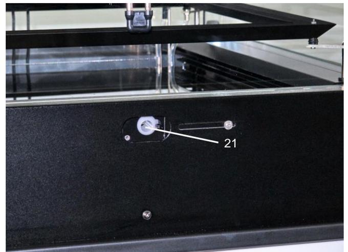
Fig. 6: Insertion for radiation sources
