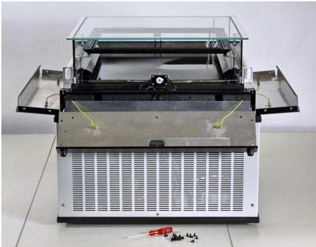
Fig. 7: Lamp change with opened cover plate
